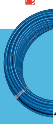
At the heart of the system is a macro composite pipe of five layers. The inside layer is made of cross-linked polyethylene (Pex). This is bonded to an overlapped welded aluminium layer which in turn is bonded to an outside cross-linked polyethylene (Pex) layer. All layers are extruded in one step. The middle aluminium layer is 100% gas/oxygen tight. This structure gives Gas Pex™ pipe the advantages of both metal and plastic while avoiding their weakness.
